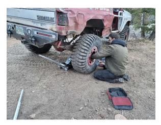
On his way out the exit of the Chutes, Nate managed to pull a tire out of the beadlock. We had to unbolt the
