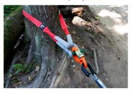
chained together make good anchor points. In sand, bury your spare tire horizontally, a foot or two deep. A buried log can make a good anchor also.
