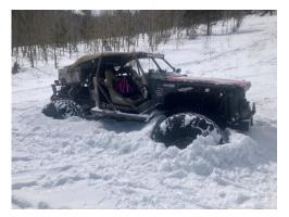
logs – anything that will support the vehicle's weight. If you do any digging replace the soil and clean up afterward. You might be able to lighten the vehicle enough to raise the chassis and allow you to pull off the obstruction. To do this take out gear, gas cans, and people. However, if you are hung on an axle, this probably won't work.
